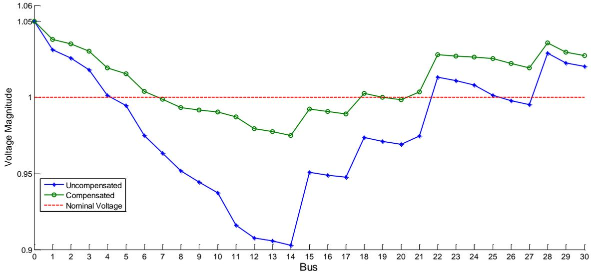
**Fig. 6. Voltage profile at peak load level for compensated and uncompensated systems at the peak load level of the present year, deterministic case.**
