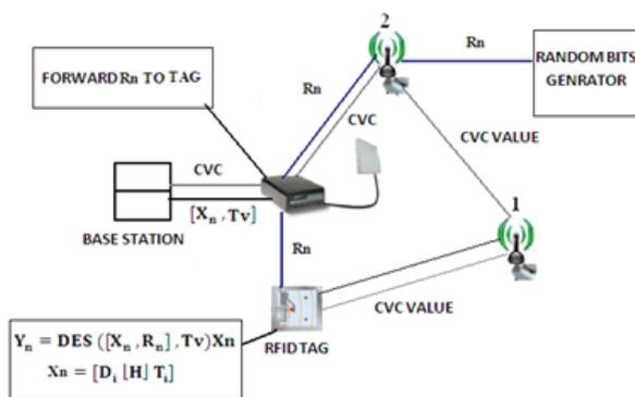
Figure 1: Proposed integrated model for RFID system
